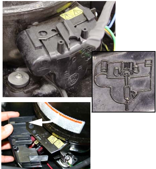
Figure 6: Access compressor overload and relay A screwdriver may be used to release the latch.
