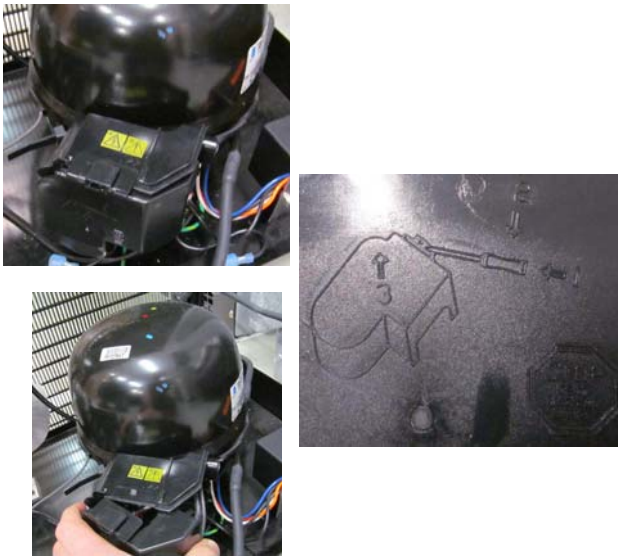
Figure 8: Access compressor overload A screwdriver may be used to release the latch.
