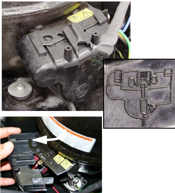
Figure 28: Access compressor overload and relay
